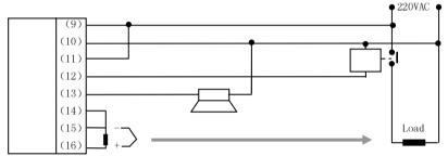
(2) Terminals for Model (with SSR): XMTD-6401V, 6401V, 6302V, 6402V and XMTF-6301V, 6401V, 6302V, (96×96) (96× 48
