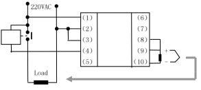
(8) Terminals for Model (with SSR): XMTG-6301V, 6401V, 6302V, 6402V(48×48)
