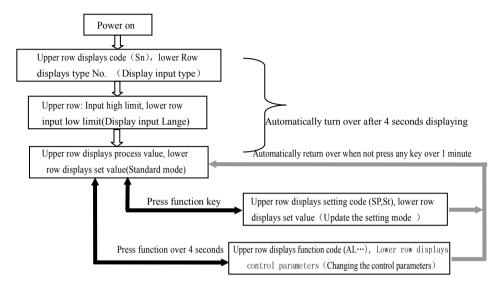
Example: Input: Thermocouple E, 0~400°C. When turn on power, display:
