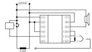
(5) Terminals for Model (with SSR): XMTE-6301V, 6401V, 6302V, 6402V(72×72)
